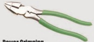
Power Crimping Combination Plier Light duty, dipped handle Material: Carbon steel, chrome-vanadium Finish: Fine polished, nickel-plated Size: 10" M.01152
